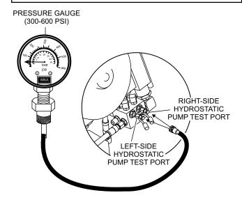
Figure 48. Steering Pressure Gauge
